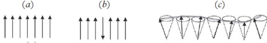
Figure 2.3: (a) All spins in a given lattice direction are aligned due to exchange interaction. (b) A single-flipped spin creates an excited state. (c) The wave-vector-dependent quantized form is called a magnon, where the spin vectors precess on the surface of cones, with a constant phase angle between successive spins that are separated by the inter-atomic lattice spacing. The figure is adapted from reference [1].
