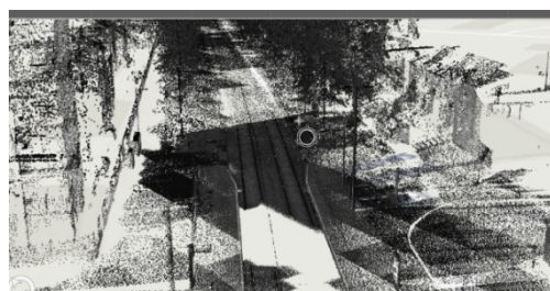
Figure 10: Point Cloud Visualised in GIS (3D Laser Mapping 2018)
