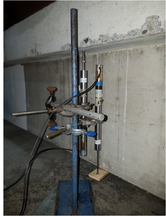
(b) LVDT to measure the displacement of the slab relative to the beam
