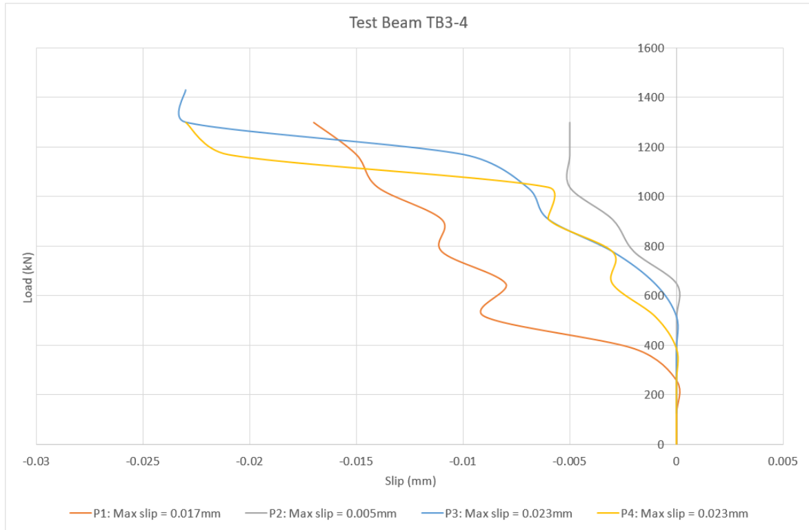
Figure 3.23: TB3-4 Graph for Beam to Slab Displacement
