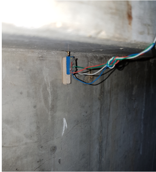
(a) View of Potentiometers positioned stuck to slab with screw touching the underside of the slab
