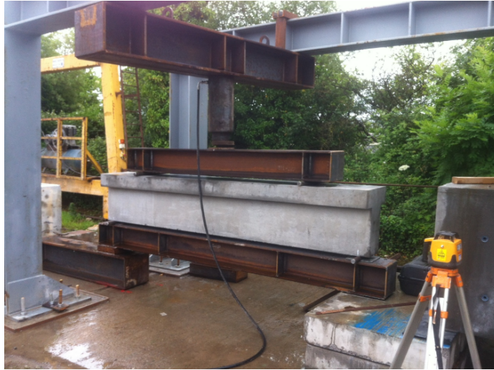
Figure 3.20: Beam Test Specimen prior to loading in Banagher Precast Concrete
