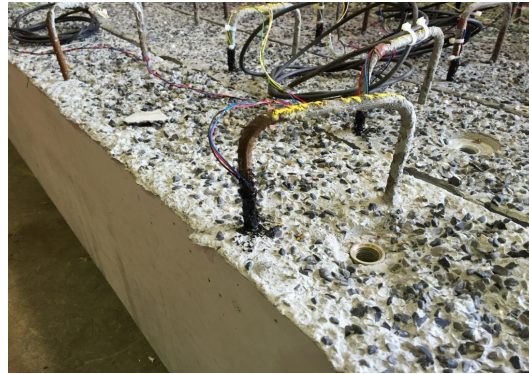
(b) Strain gauge positioned on stirrup of TB4-3 just above the interface and protected with black silicon
