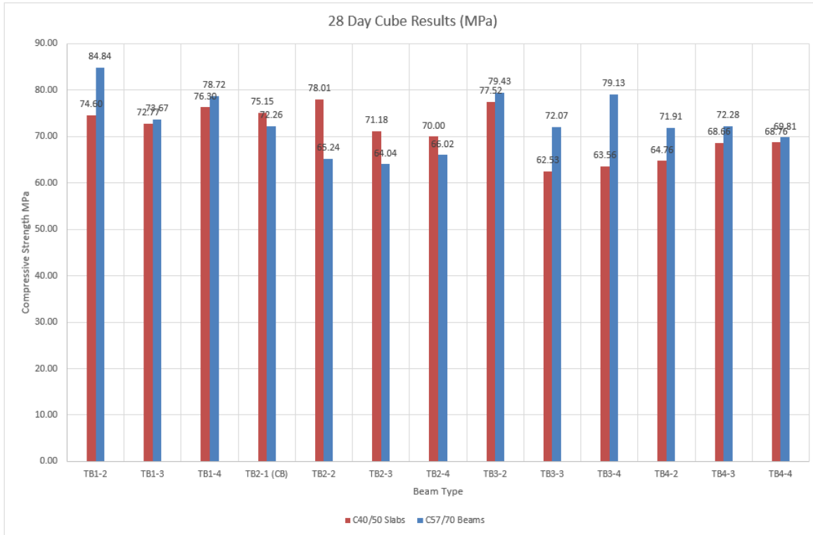
Figure 3.6: Phase 1 28-day compressive strength
