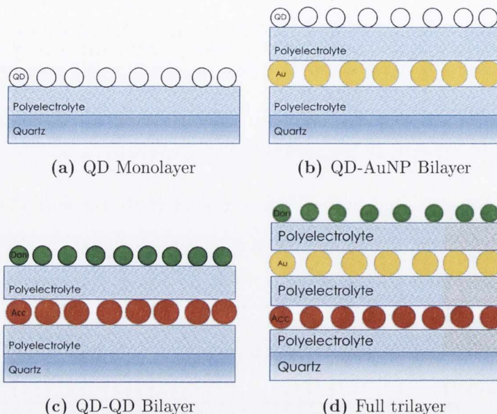
Figure 3.3: Schematic of the structures used in the temperature dependent studies. (a) Monolayer of either donor or acceptor QDs with varying concentrations. (b) Separated bilayer of AuNPs and a densely packed monolayer of either donor or acceptor QDs with a 3 nm PE spacer layer. (c) Separated bilayer of donor and acceptor layers (densely packed) with a 3 nm PE spacer layer (d) Schematic of the full trilayer sample.
