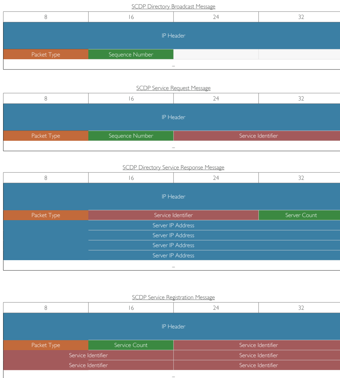
Fig. 4.14: SCDP uses 4 protocol message types, allowing directories to advertise their presence, service agents to register their services and user agents to request services either by directly querying directory nodes or by broadcasting.
