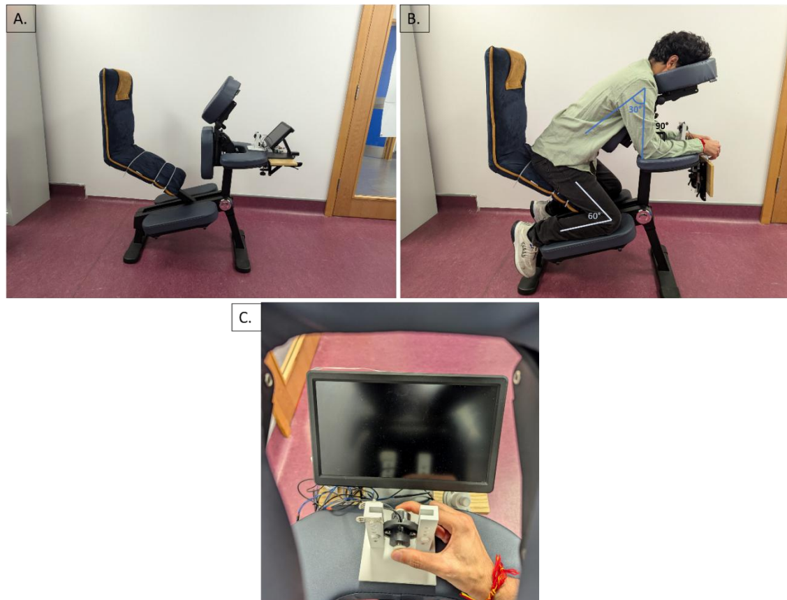
Figure 22: A. The setup with the physio-chair and 10.1-inch screen that was used during the experiment. B. A participant sitting in an inclined position on the physio-chair. The participant's chest was supported by the chest rest while their head rested on the headrest and hands rested on the handrest respectively. C. The photo demonstrates the hand position during the voluntary motor task. The photo also showcases the force sensor system and the 10.1-inch screen used during the task, from the perspective of the participant (photo taken through headrest).
