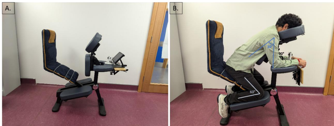
Figure 10: A. The setup with the physio-chair and 10.1-inch screen that was used during the experiment. B. A participant sitting in an inclined position on the physio-chair. The participant's chest was supported by the chest rest while their head rested on the headrest and hands rested on the handrest respectively.
