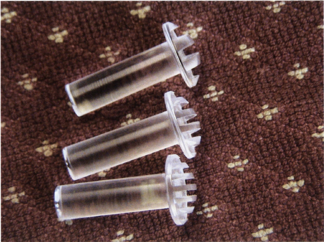
A selection of Johnson-Van Boven-Phillips domes (scale approx magnified x2), showing the acrylic dome shaped heads with grooves and ridges of equal width
