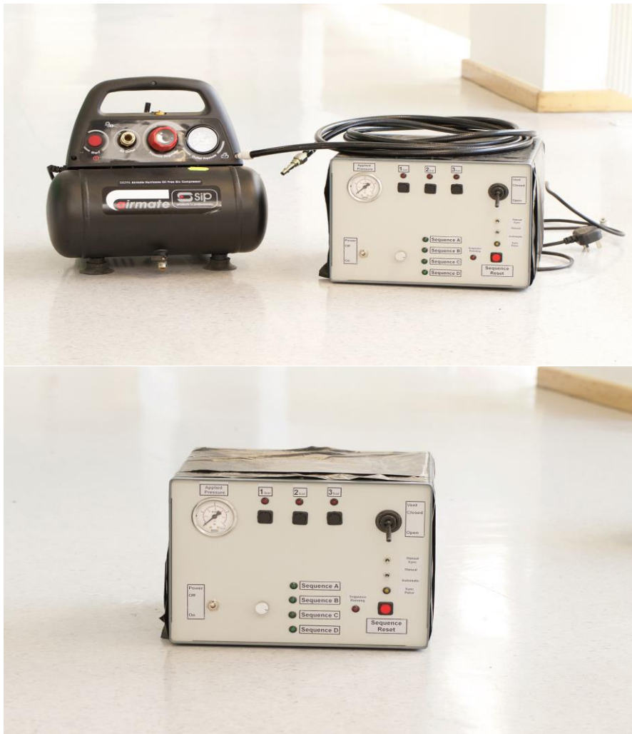
Figure 3. The custom-built pressure algometer and air compressor.
