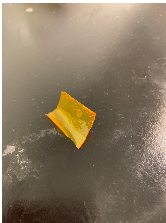
Figure 3.10 Image of drop casting fabricated LDS layer.
