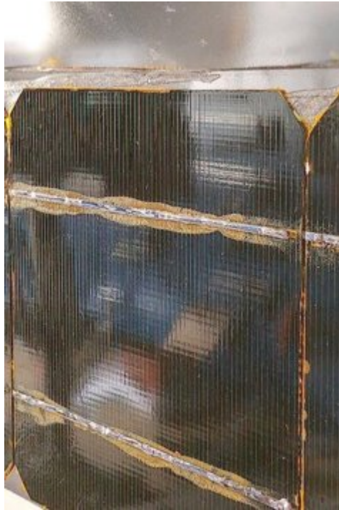
Figure 6.5 Image of soldering's effect on LDS
