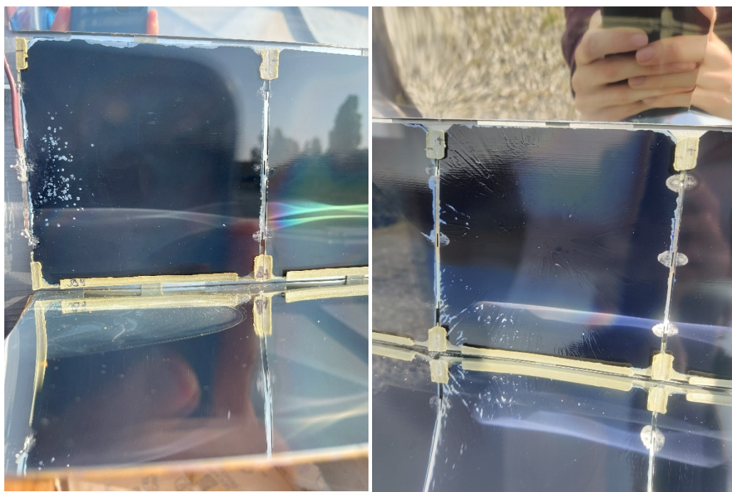
Figure 6.16 (A) & (B) Examples of layer decay and non-uniformity occurring
