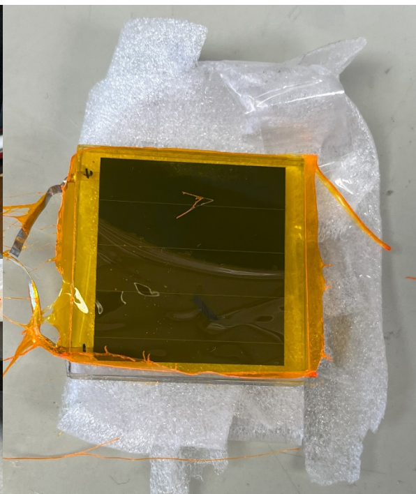
Figure 7.3 (B) close up of LDS on CdTe
