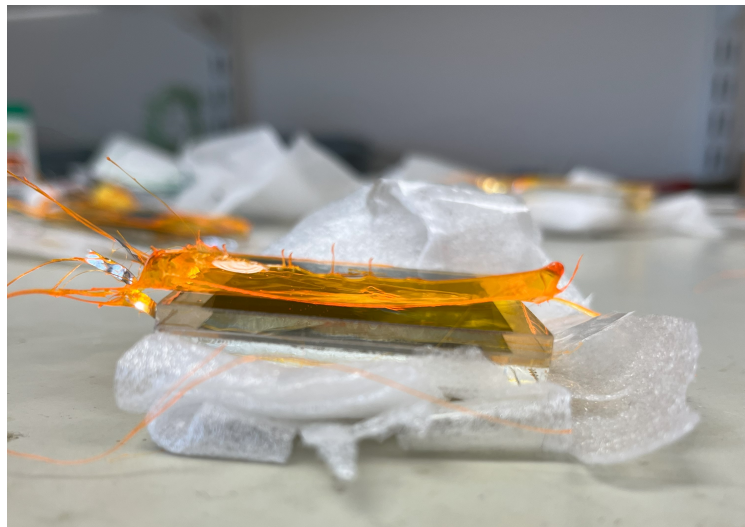
Figure 7.4 Image of LDS layer peeling from CdTe cell surface.
