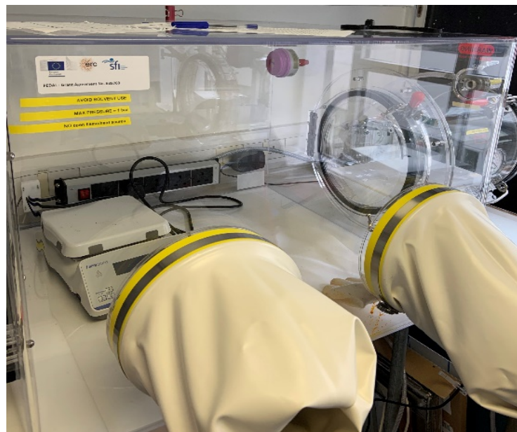
Figure 3.14 Image of Nitrogen Glove box in Watts lab
