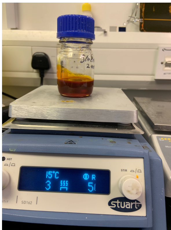
Figure 3.2 Magnetic stirrer hot plate. Note the heat function was turned off.
