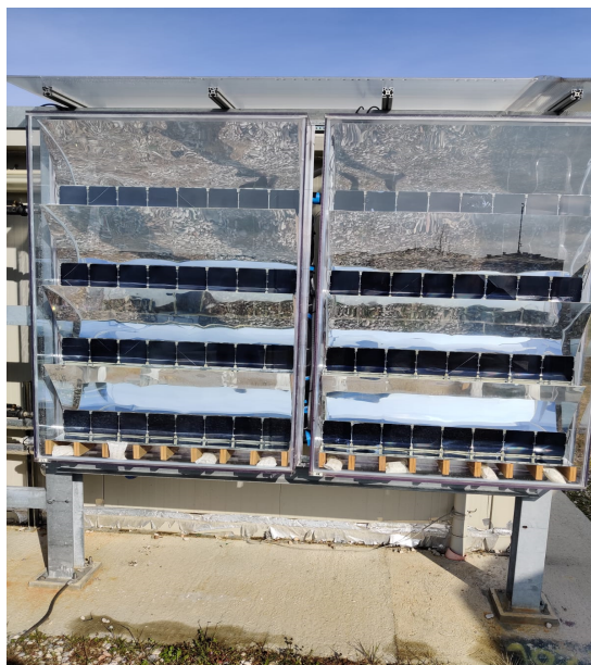
Figure 6.15 LDS layer PV integrated CPC systems at Site 1 in Ferrara, Italy.
