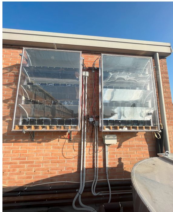
Figure 6.21 2 nd set of LDS coated CPC systems used at test site on UNIFE campus in Ferrara.
