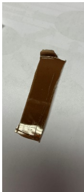
Figure 7.9 Sample cut to the size of sample holder; 2 cm wide and 5 cm long.
