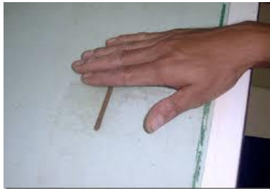
Thread-rolling method (Atterberg)
