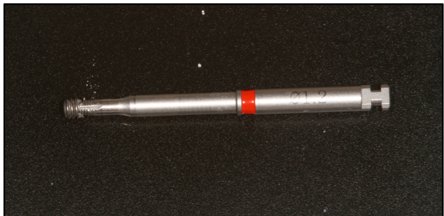
Figure 52: The Screw Remover SR12 with a basal screw fragment attached
