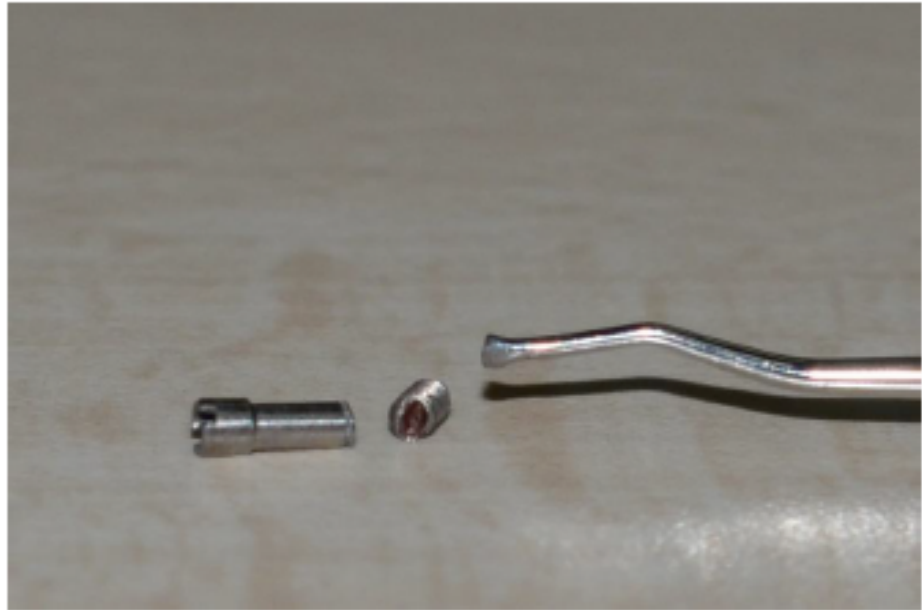
Figure 6: An example of instrument modification: a spoon excavator has been modified by cutting the working end of the instrument perpendicularly to create fork shape, allowing it to engage the fractured screw fragment. Adapted from Satwalekar et al. (2013) (104).
