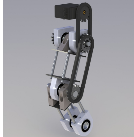
Figure 2.5 Drive System of the Knee Joint
