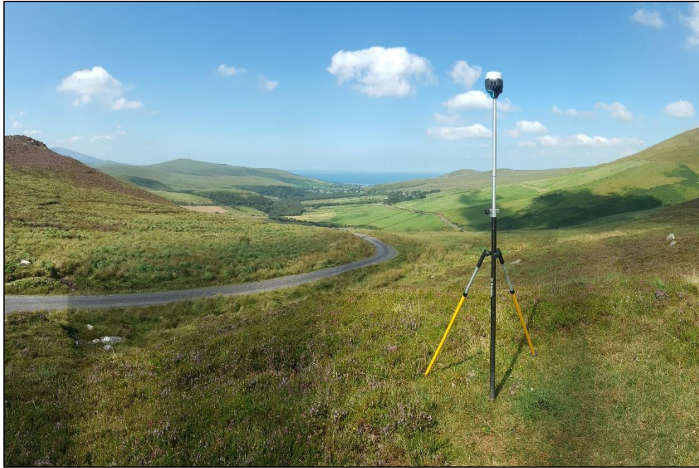
Figure A.13. A GNSS receiver recording the coordinates of a training point in Slieve Mish, Co. Kerry.
