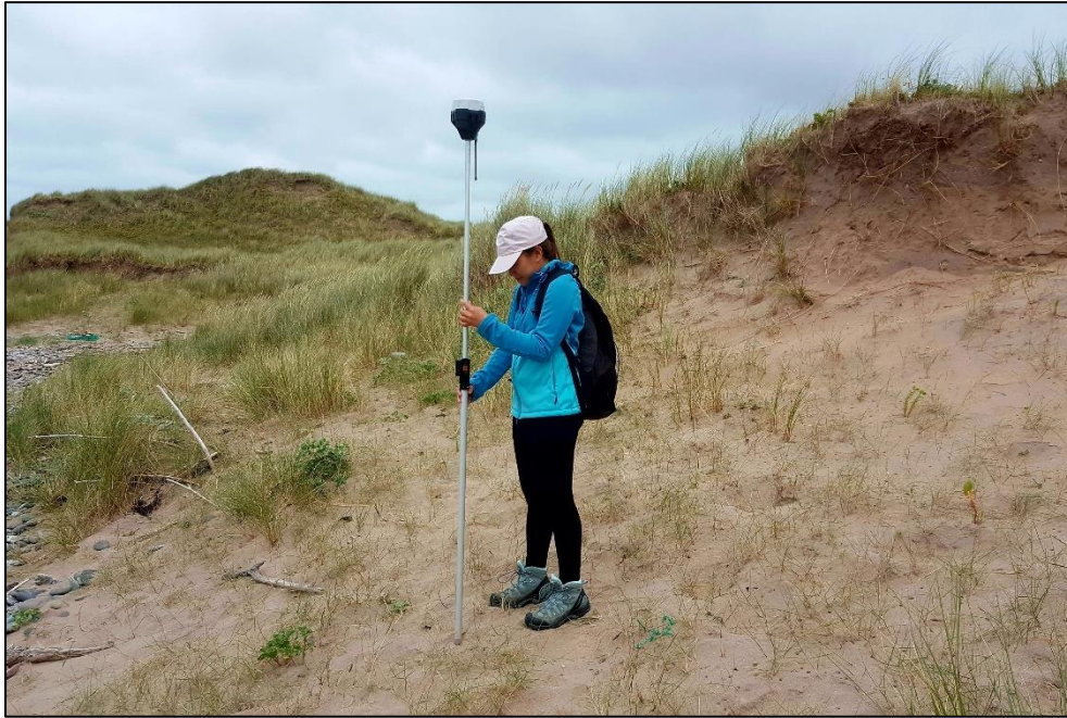
Figure A.11. C. Cruz measuring the coordinates of a training point using a GNSS receiver.
