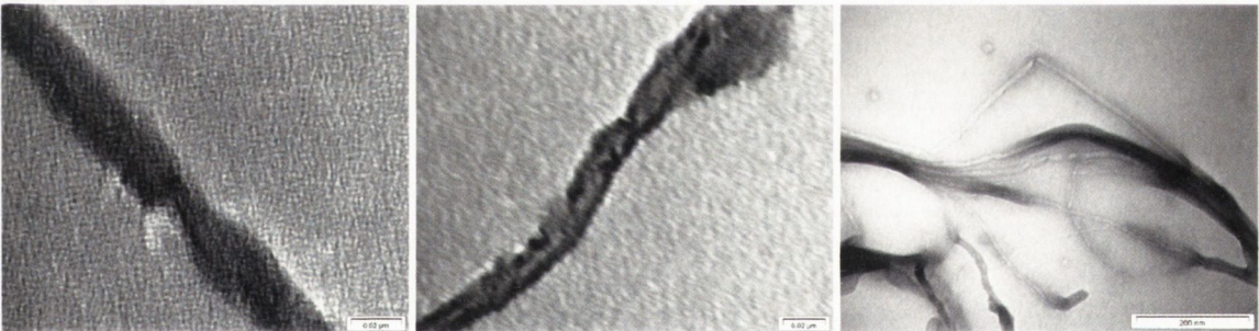
Figure 5-27: Transmission electron microscopy images of thin multi walled carbon nanotubes covered with chemically bonded chlorinated polypropylene
