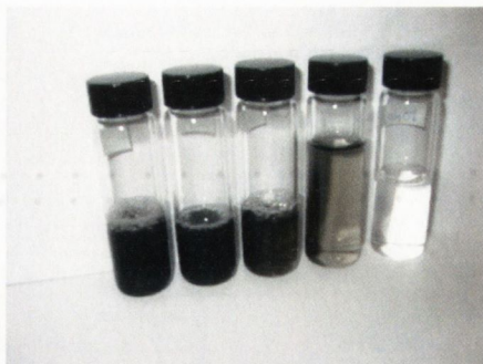
Figure 3-28: Sample bottles of blended range of polyvinyl alcohol/ carbon nanotube solutions (Foam appears after sonification. Solution is for a long term stable)
