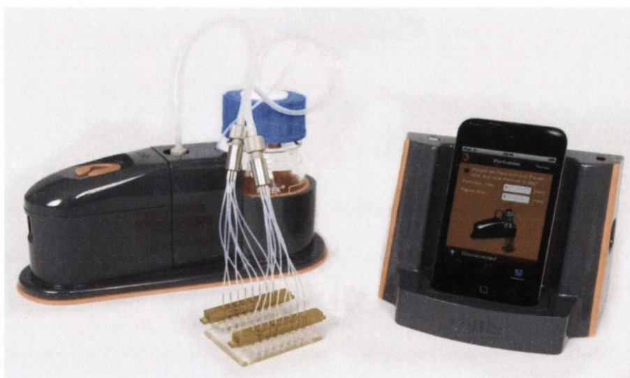
Figure 3.3 iKima pump App 1. Set-up -Select iKima App on iPod Touch or iPhone. Connect iPod Touch to iKima controller: Press "Connect" button. 2. Wash out- Select "wash out" button 3. Flow assay- The user can select two flow rates for two different time periods. These two flow rates are then continuously looped or cycled until the user stops the device
