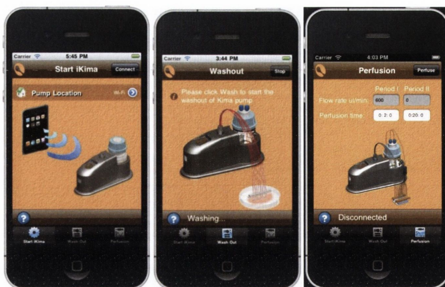
Figure 3.3 iKima pump App 1. Set-up -Select iKima App on iPod Touch or iPhone. Connect iPod Touch to iKima controller: Press "Connect" button. 2. Wash out- Select "wash out" button 3. Flow assay- The user can select two flow rates for two different time periods. These two flow rates are then continuously looped or cycled until the user stops the device
