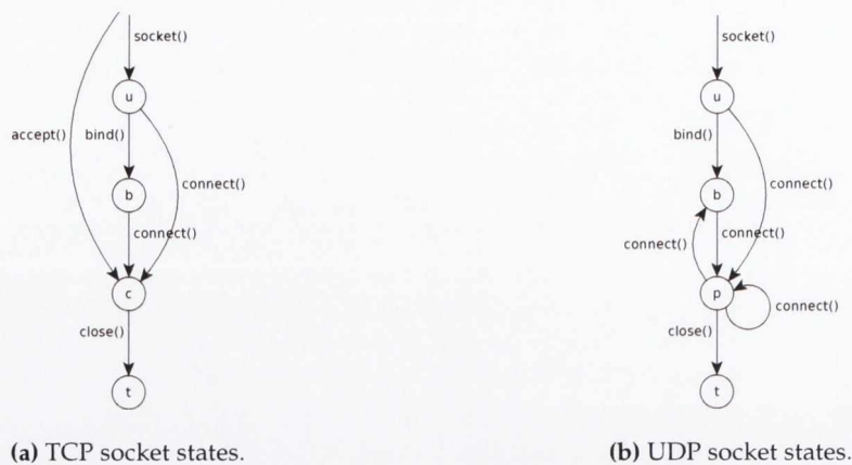
Figure 4.8: TCP/IP socket states. For the two types of sockets—TCP or UDP—the possible states are: u —the unbound state, where the socket is created but has not been assigned an EID yet; b —the bound state, where an EID has been assigned to it, but no peer is bound yet; a —the associated state, where the socket is bound to its own EID and associated with its apposite’s EID and state (only relevant for TCP/IP); t —the terminated state, after the socket is closed.
