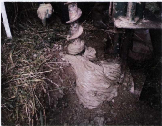
Figure 5.9 Material encountered 5.5 m b.g.l at piezometer 1b at the fractured-volcanic poorly-drained arable (FvPDa) site during Gidding’s Rig drilling.
