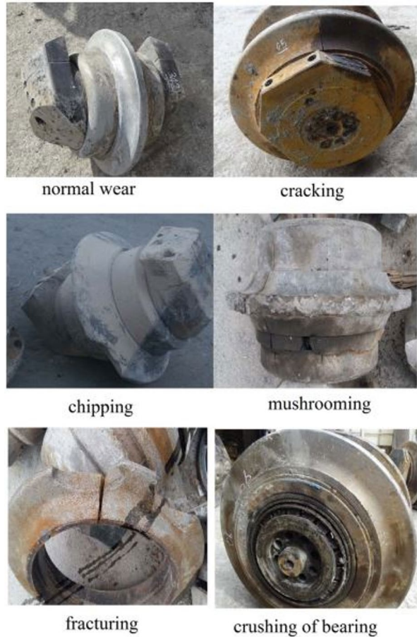
Fig. 4 Examples of disc-cutter failure patterns for the KSWCT project (Sabri et al. 2023)
