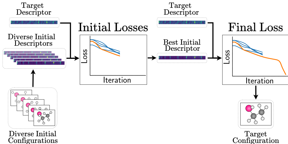
Figure 4.1: Diagram of the workflow of the proposed inversion method. It is desired to find the configuration that corresponds to some target descriptors. The maximally diverse configurations from a molecular dynamics trajectory are used as initial guesses. At each iteration, the positions of the initial configuration are updated, see Equation (4.2), so as to minimise the difference between the target descriptors and the initial descriptors, see Equation (4.1). After N_{init} iterations, the initial configuration with the lowest loss is selected, and the procedure is continued for a total of N_{iter} iterations. If convergence is reached, the resulting target configuration has been updated sufficiently that its descriptors are approximately equal to target descriptors. Therefore, the target descriptor has been inverted, with an appropriate configuration found.
