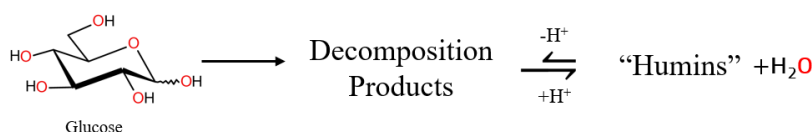
Figure 8. Proposed reaction scheme for the formation of humins from lignocellulosic biomass.
