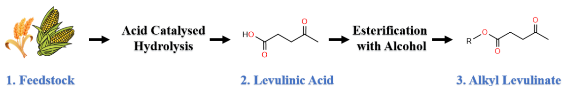
Figure 17. Schematic of the two-step hydrolysis–esterification pathway for producing alkyl levulinates from lignocellulosic biomass. Carbohydrates are first converted to levulinic acid via acid-catalysed hydrolysis, followed by esterification with an alcohol to yield the target alkyl levulinate. This route requires sequential processing, making it slower and less atom-economical than alcoholysis.
