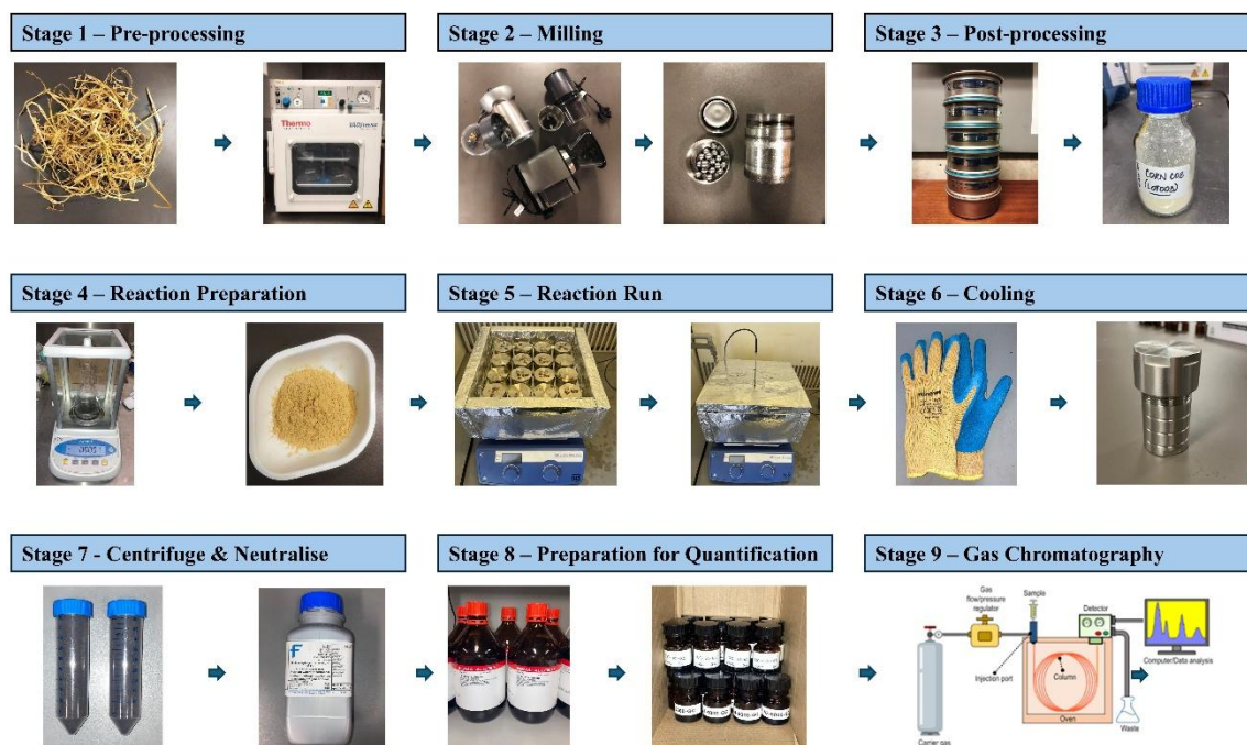
Figure 19. Overview of the nine-stage experimental workflow, from biomass preprocessing and milling through reaction preparation, reaction run, cooling, centrifugation, and sample preparation, concluding with product quantification by gas chromatography.
