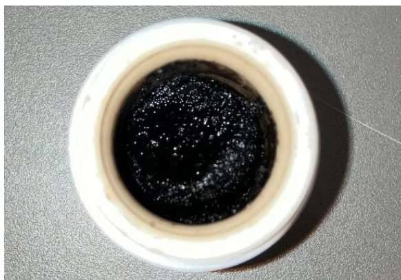
Figure 44. Solidification of the xylan reaction mixture during acid-catalysed butanolysis at 20 wt.% loading after 3 h at 170 °C.
