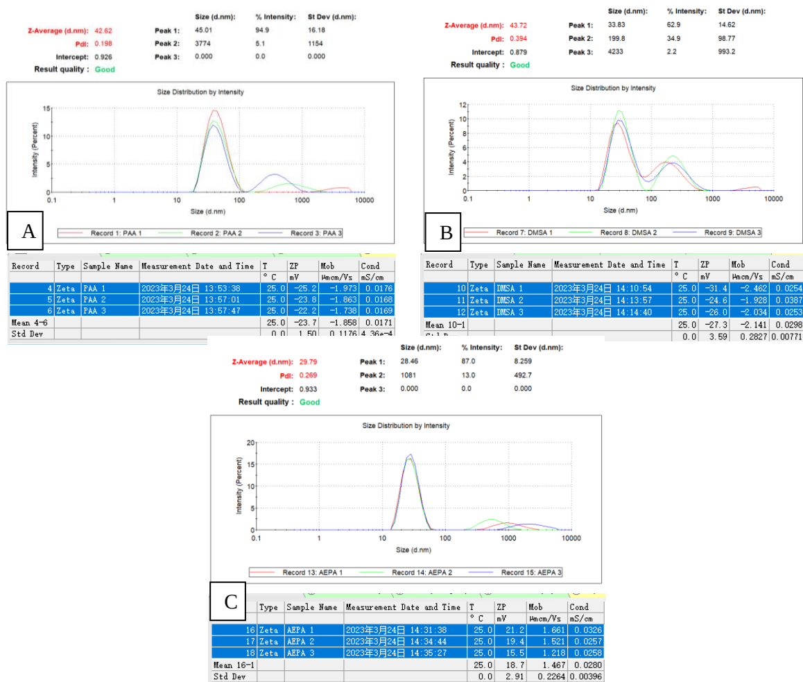
Figure 15: The size of the three developed MNPs in water were tested at a concentration of 300 μg/ml, following 30 minutes sonication and filtration. The MNPs included PAA (A), DMSA-MNPs (B), and AEPA-MNPs (C).
