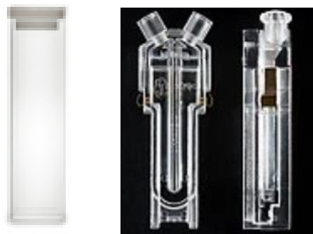
Figure 5: Square glass cell used for DLS (PCS8501, left) and disposable folded capillary cell used for ELS (DTS1070, right).
