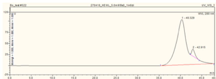
Figure 9. Size-exclusion chromatogram of a mixture of cross-linked HEWL (trimer, dimer, monomer)
