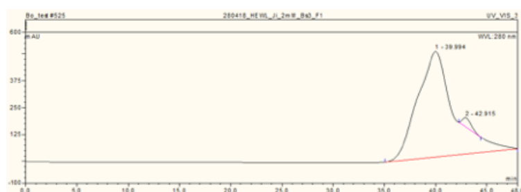
Figure 10. Size-exclusion chromatogram of mixture of cross-linked HEWL (trimer & dimer enriched via centrifugal concentration)
