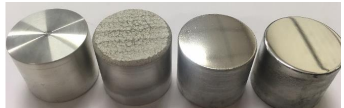
Figure 2: Substrate, cold sprayed sample, polished sample and buffered sample (left to right)
