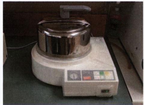
Fig 3.21. Acrylic packed to form stent and cured under heat and pressure.
