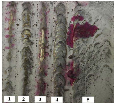
(a) Dye penetrant inspection of LC coatings
