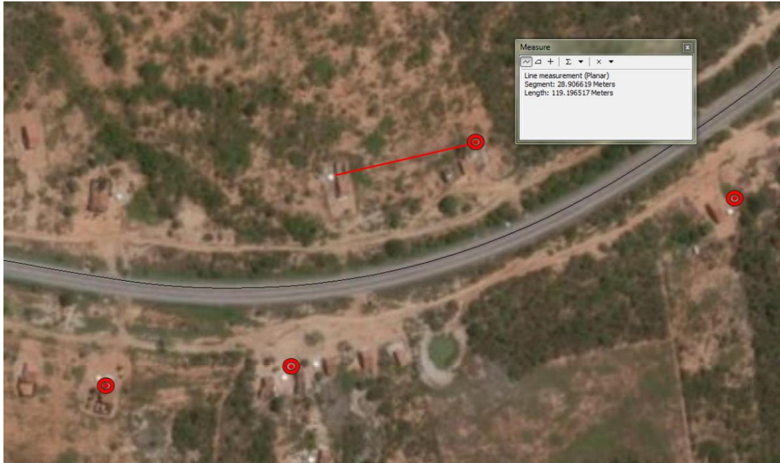
Figure 3.9: Sample of accuracy checking of cisterns location (screenshot taken from ArcMap 10.6.1)
