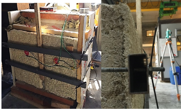
Fig. 2. Hot-box assemblage for thermal conductivity measurement.
