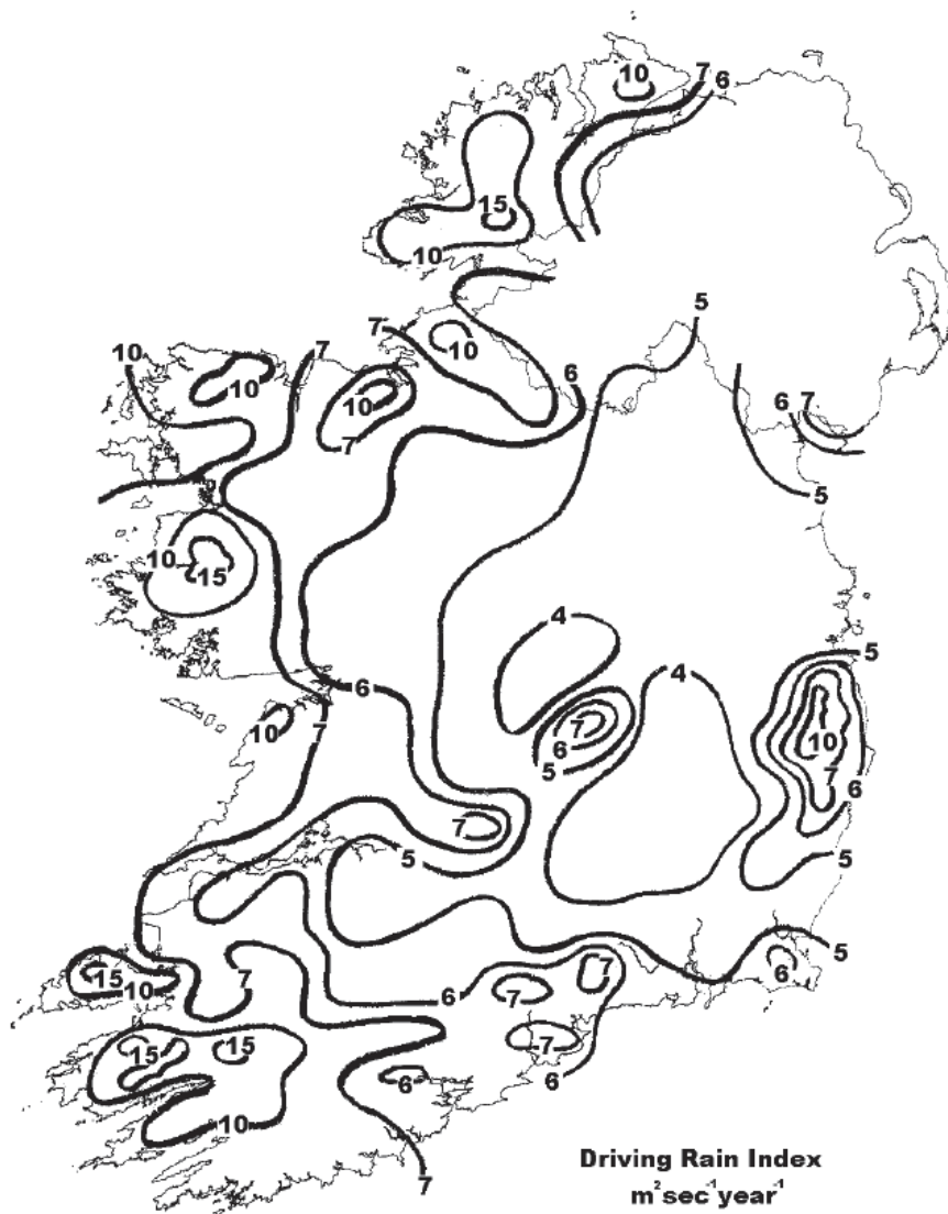
Figure 4: Driving Rain Index Map of Ireland, courtesy of the Report of the Expert Panel on Concrete Blocks, 2017.
