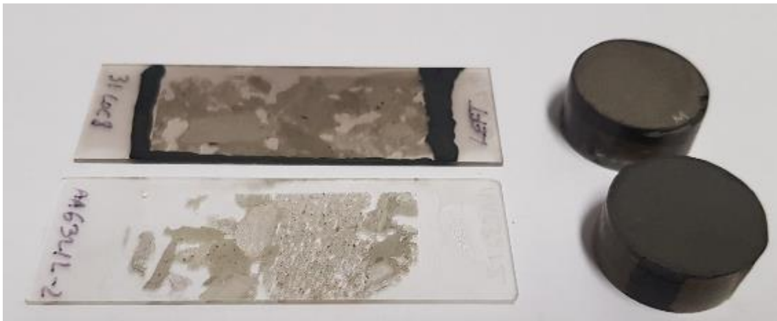
Figure 6: Polished thin sections of concrete blocks on the left (carbon coated to the rear, the boundary painted with colloidal graphite) and two polished round one inch pucks of sand embedded in resin, with a narrow rim and side strip of colloidal graphite applied.
