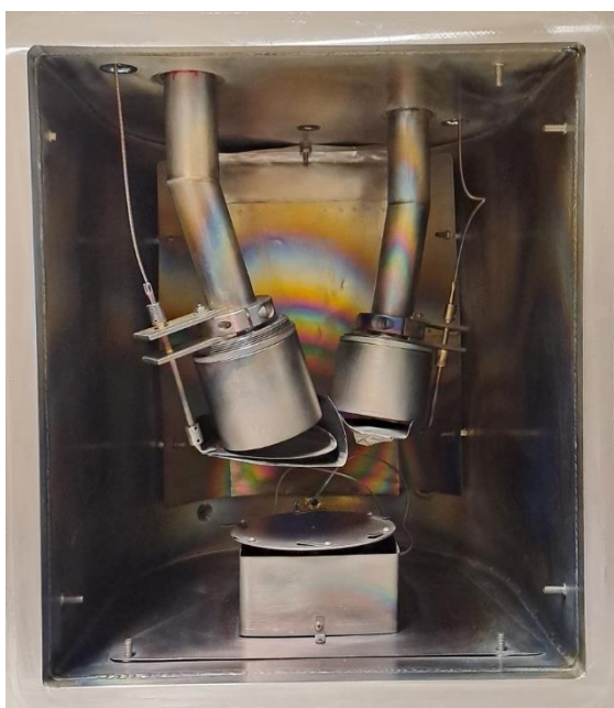
Figure 2.2 Sputter chamber used for deposition of carbon and metal films.
