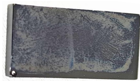
Figure 4.2 Image of MoS 2 grown on an-C:N Graphitic on a GC plate (2×1 cm 2 ) used for electrolysis.
