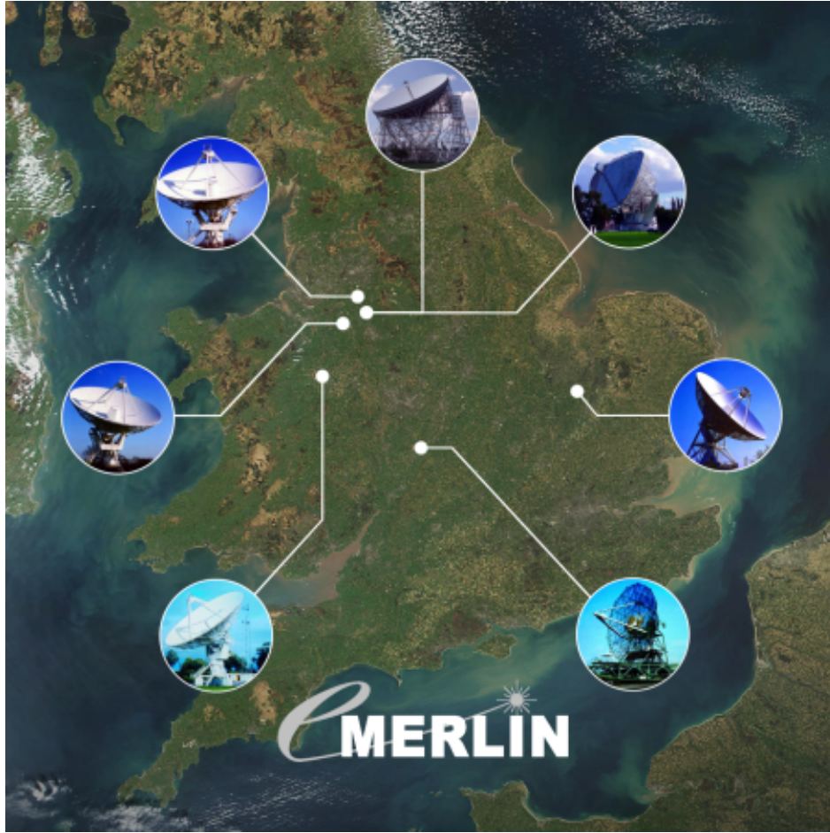
Figure 3.8.: e-MERLIN is an array of radio telescopes distributed around Great Britain, with baseline separations of up to 217 km. Image credit: www.e-merlin.ac.uk .
