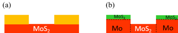
Fig. 3.11: (a) Standard top contact design (b) Phase engineered contacts by co-sulphurising bulk Mo along with thin Mo to form a thin film MoS 2 channel (middle red box) transitioning into metallic Mo phase whose topmost layers only form MoS 2 (green).
