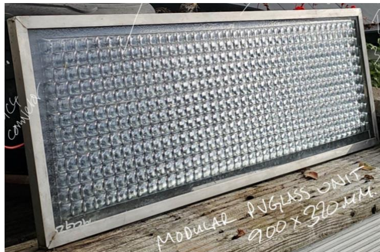
Figure 3. 7 900 x 320mm Modular unit PVGlass with flexible solar panel behind 50 W
