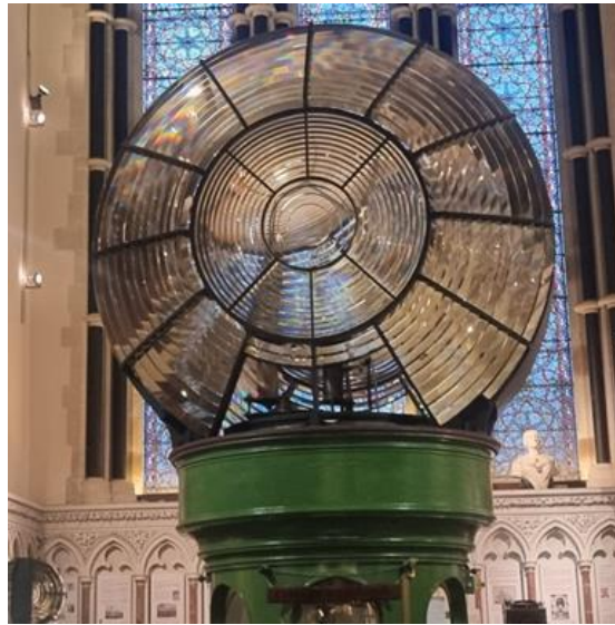
Figure 1. 7 Fresnel Lens, Bailey Lighthouse
