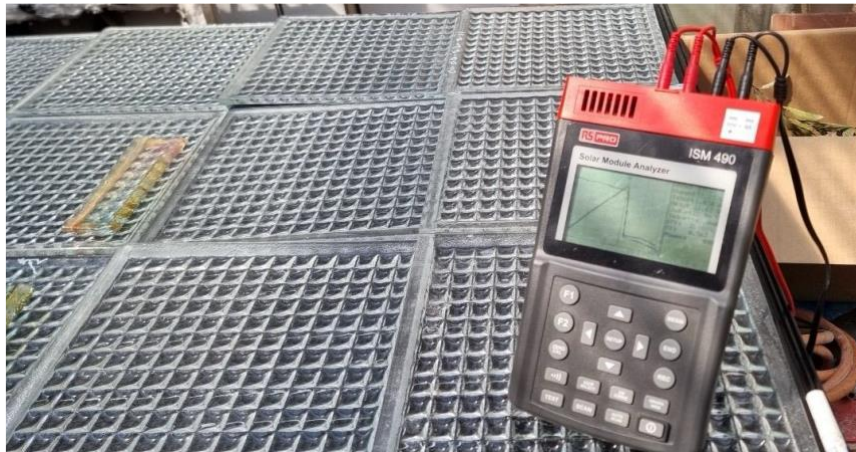
Figure 3. 4 Solar Module Analyzer connected to test panels
