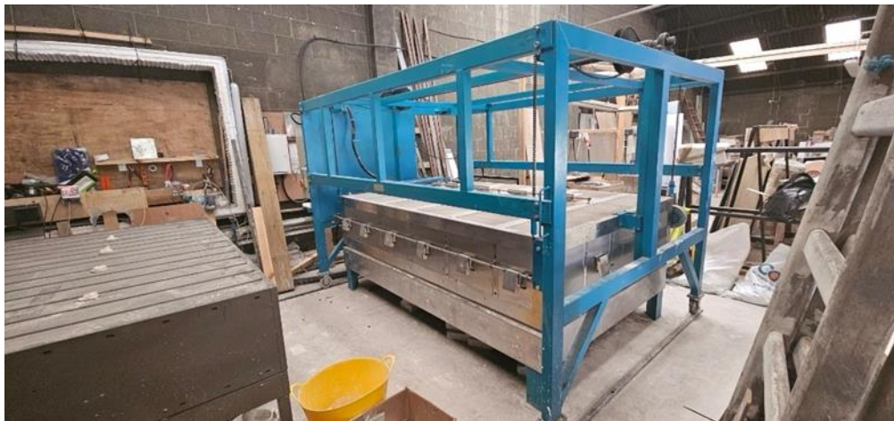
Figure 3. 1 Electric Kiln equipment for casting glass panels
