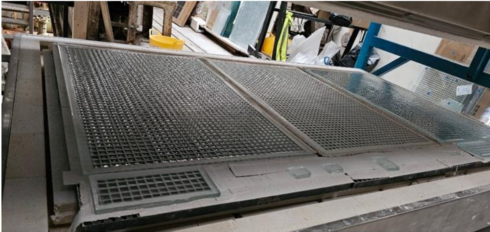
Figure 3. 2 Inside Electric Kiln, glass casting into steel moulds
