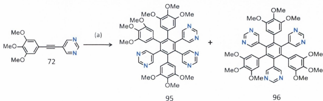
Scheme 3.8: Synthetic route to 6N polyphenylenes 95 and 96 ; (a) \text{Co}_2(\text{CO})_8 , dioxane, 115 °C, 24 h, under \text{N}_2 .
