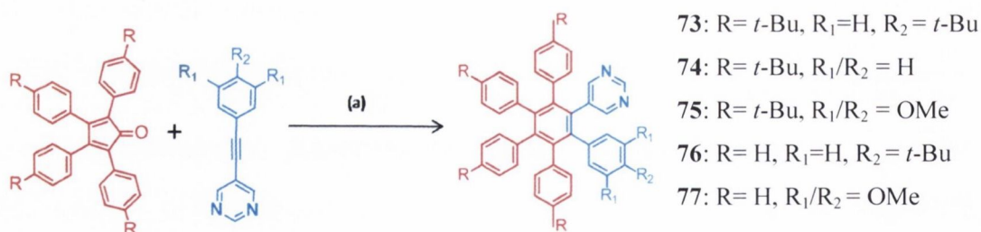
Scheme 2.2: [2+4]-Diels-Alder route to 2N polyphenylene precursors; (a) benzophenone, 280-300 °C, 2hrs, under Ar.
