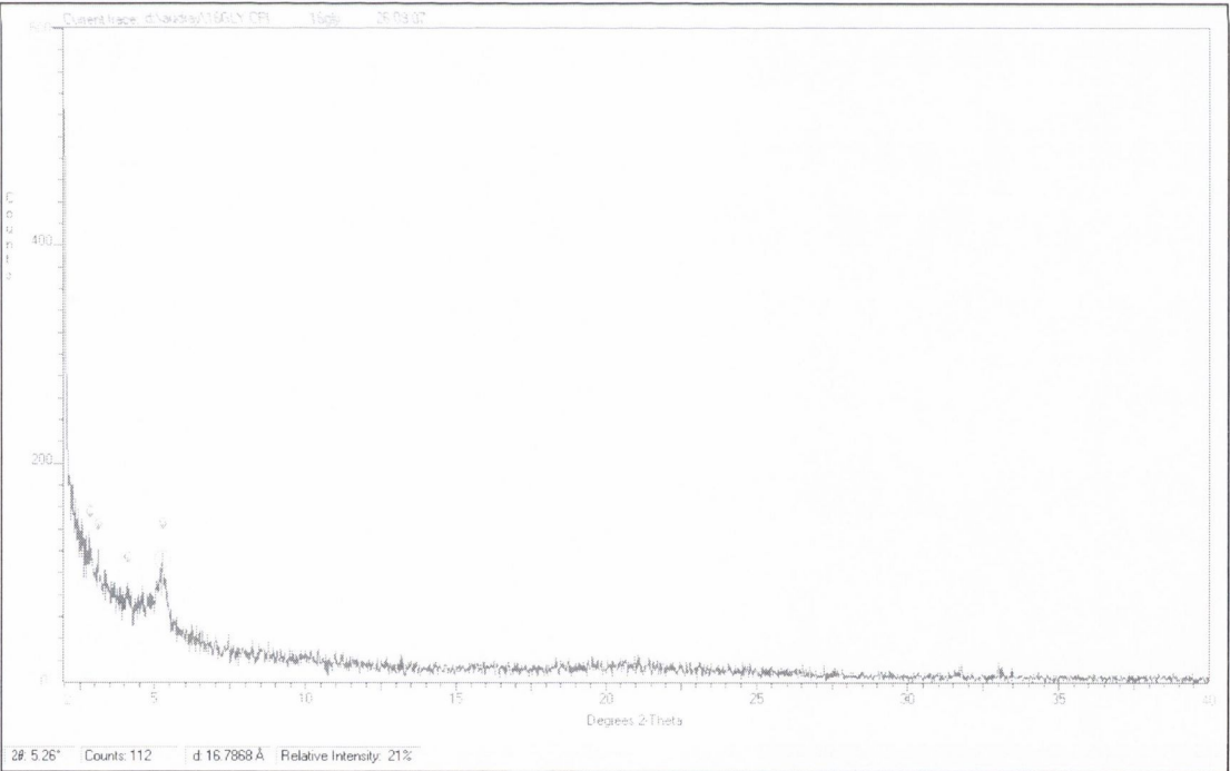
Figure 5B: XRD graph for the sample TF-G2-CR-AK; clay separation using glycol.
