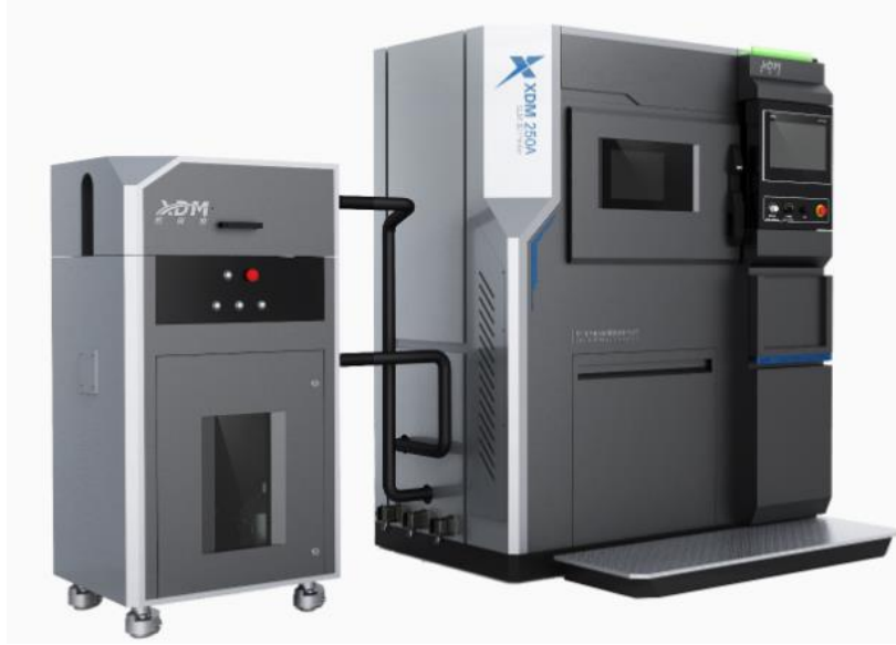
Fig. 4.2 The XDM 250 LPBF system used for high-power laser experiments.
