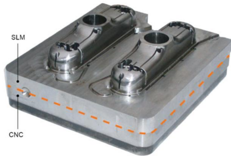
Fig. 2.6. Hybrid construction of the impression block by LPBF and CNC[32].
