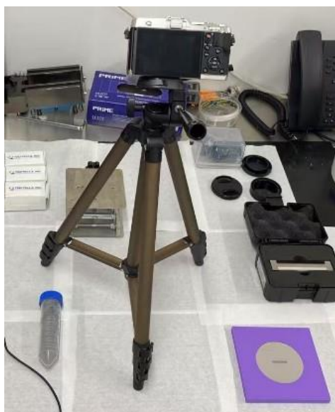
Fig. 4.4. Experimental setup for post-scan powder spatter imaging.
