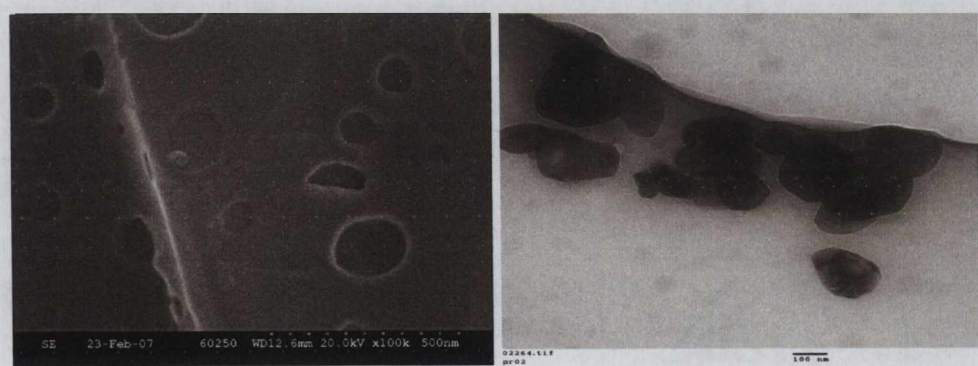
Figure 6.4 SEM (left) and TEM(right) micrographs of perylene red drop cast onto silicon (111) wafer and SiN grid respectively from a spectrophotometric grade chloroform solution
