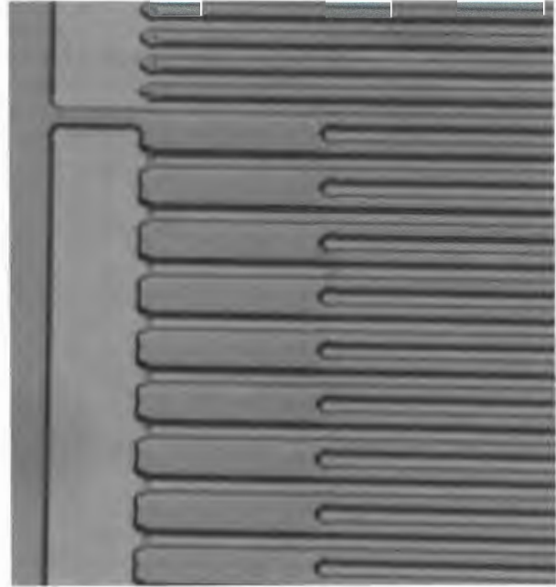
Fig. 6. Resist pattern of grating section
