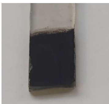
Figure 2.5.1: Film of Co@C-500/FTO after heat treatment at 500 °C.
