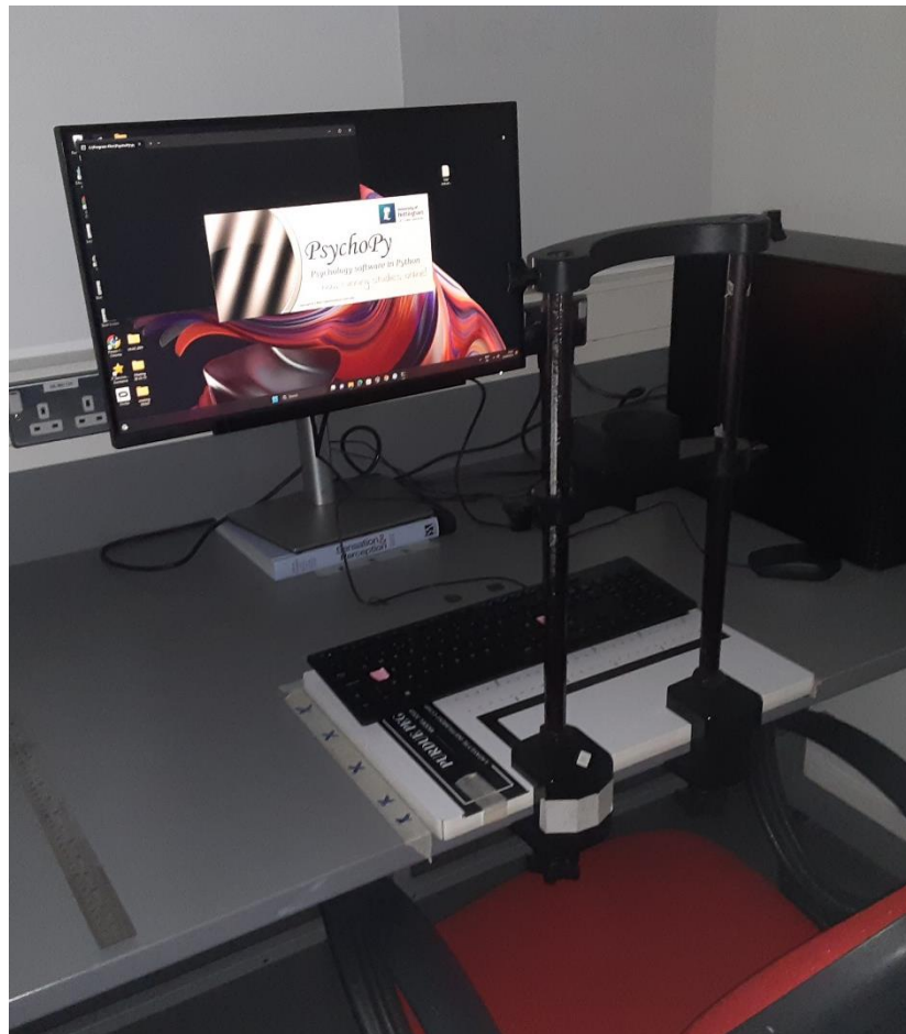
Figure 3-1: Eye tracker apparatus set up in the testing lab. Participants were seated with their heads placed in the headrest for stability throughout the course of the experiment. The Tobii Pro Fusion eye tracker was placed at the bottom of the monitor screen to record during testing.
