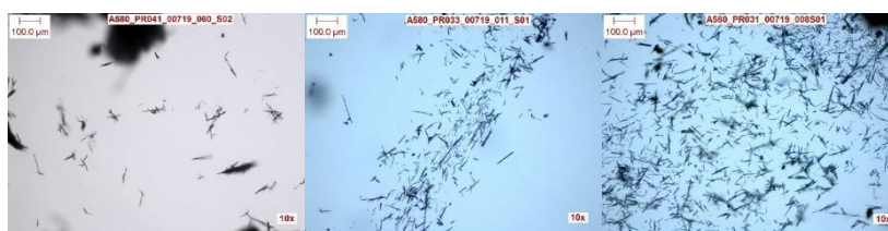
Figure 3.45: Light microscopy images of CBZ dihydrate of differing particle sizes: Small crystals (left), Medium crystals (middle) and Large crystals (right).
