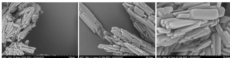
Figure 5.53: SEM images of wet THEO monohydrate with gold sputtering.
