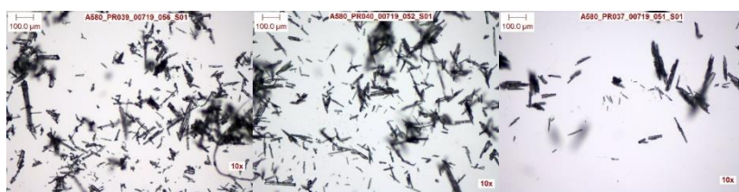
Figure 3.49: Light microscopy images of THEO monohydrate of differing particles sizes; Small crystals (left), Medium crystals (middle) and Large crystals (right).
