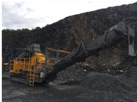
Figure 3.3 Aggregate crushing machine
