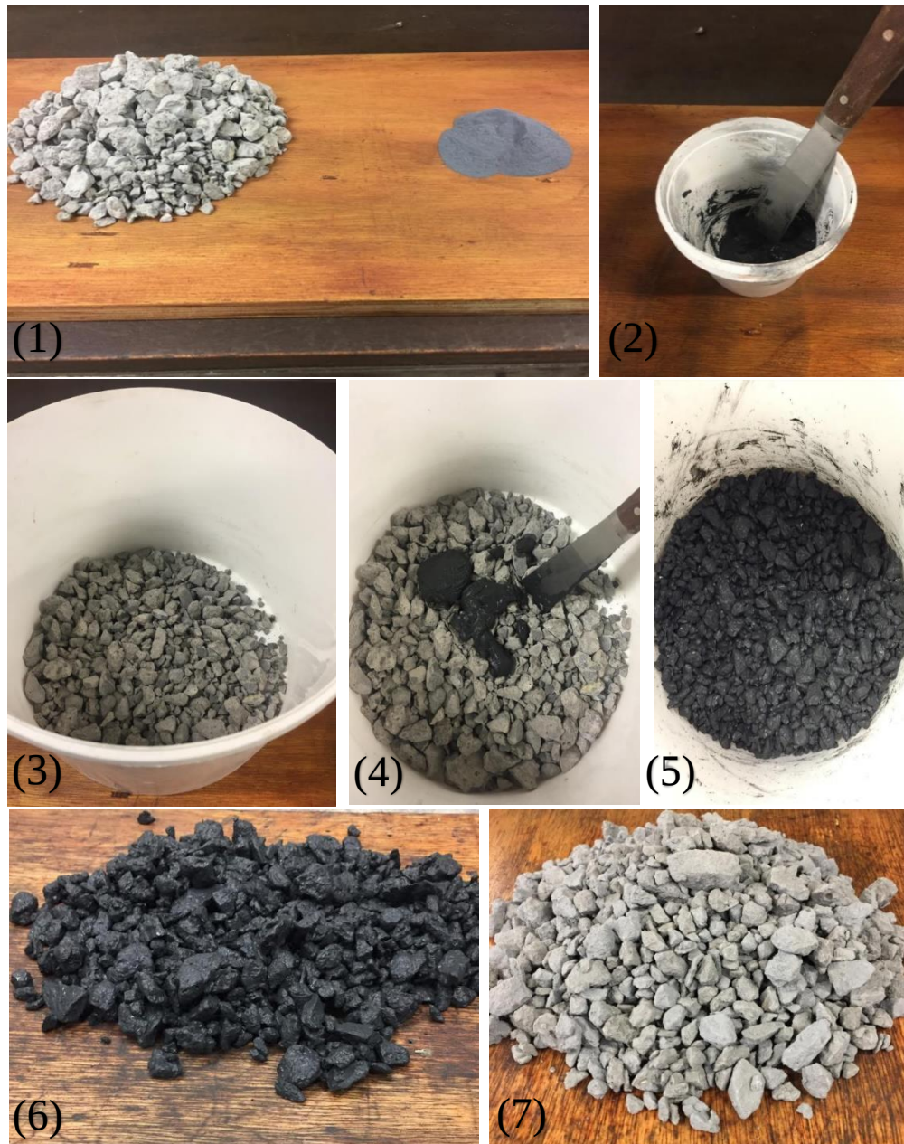
Figure 6.6 The steps of coating recycled aggregates with silica fume (1) dried aggregates, (2) preparing SF, (3,4,5) coating RCA with SF, (6) leaving the coated RCA to dry, (7) final product
