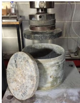
Figure 5.5 California bearing ratio (CBR) testing apparatus
