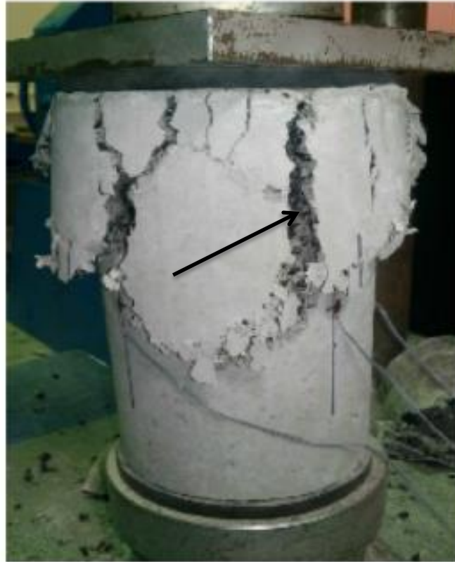
Figure 2.7 Large transverse deflection observed in rubberized concrete specimens with 100% rubber content (Miller and Tehrani, 2017)
