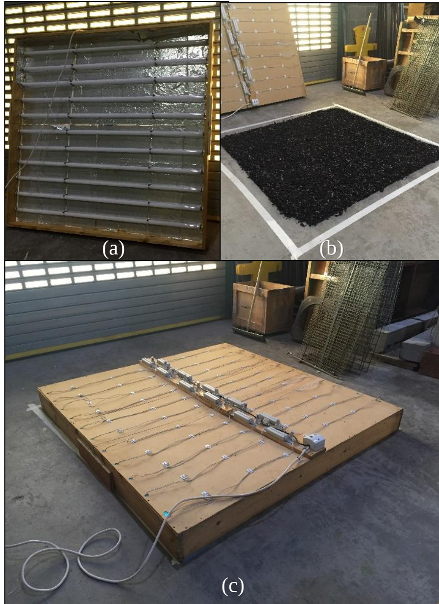
Figure 5.3 (a) ultraviolet light tubes. (b) chipped rubber aggregates (c) ultraviolet light box on the rubber aggregates
