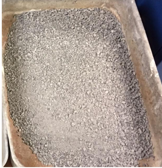
Figure 6.10 Fine recycled concrete aggregate (recycled sand)
