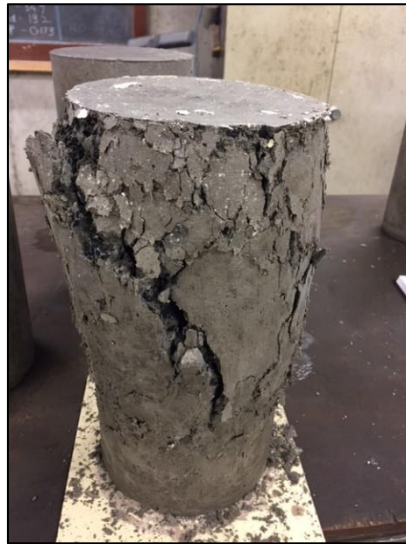
Figure 5.12 Rubber aggregate concrete cylinder's failure type
