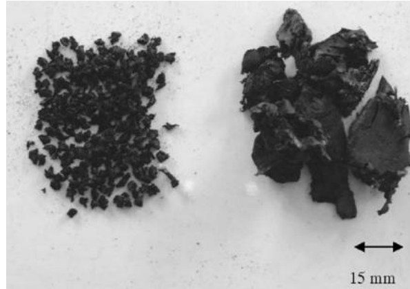
Figure 2.2 (a) crumb rubber, (b) chipped rubber particles (Khaloo et al., 2008)
