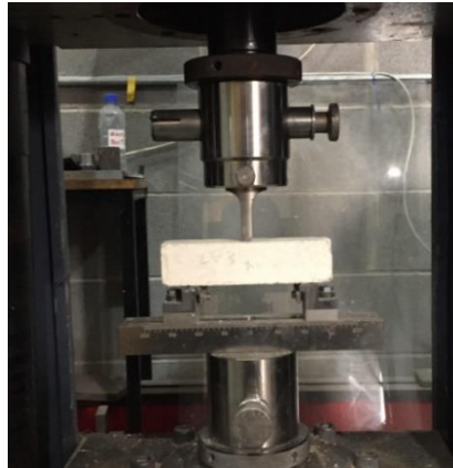
Figure 6.14 Prisms flexural test
