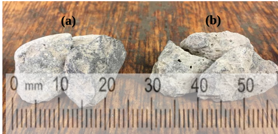
Figure 6.2 a) normal aggregates, b) recycled concrete aggregates
