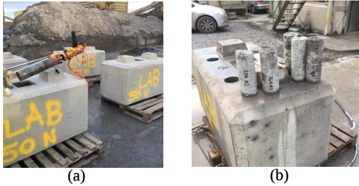
Figure 3.2 (a) Kelly blocks, (b) Concrete cores
