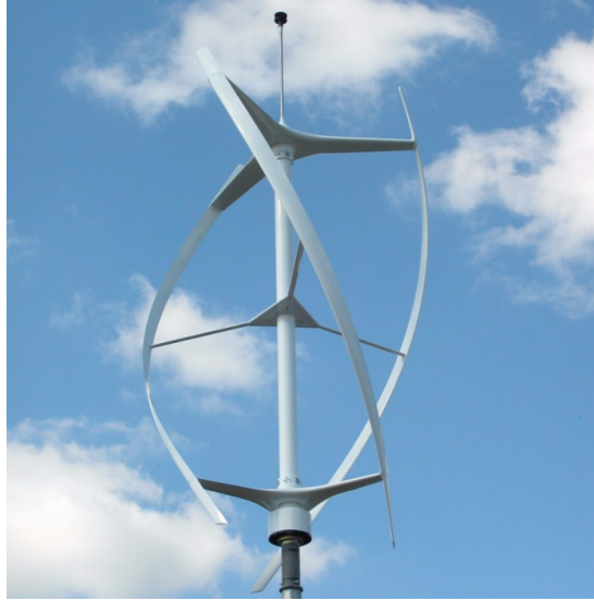
Figure 4.3: QR5 vertical axis wind turbine in operation [128].
