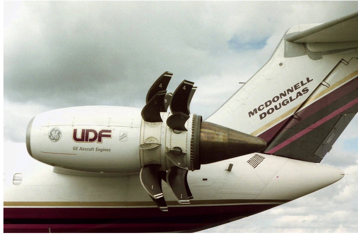
Figure 1.2: General Electric contra rotating open rotor as seen at Farnborough, 1988 [19].
