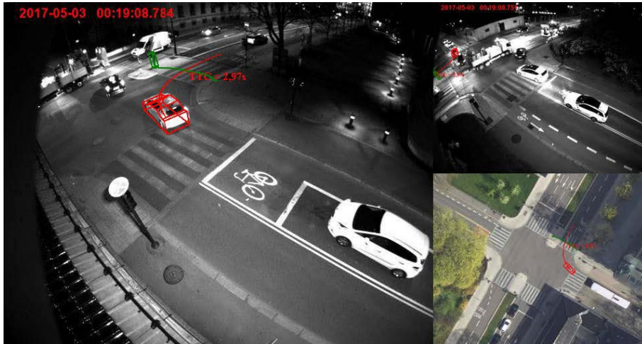
Figure 2.5: T-Analyst software for road user trajectory tracking. Figure from Johnsson et al. (2021) [62].
