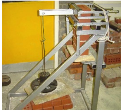
Fig. 2 Bond strength test set up
