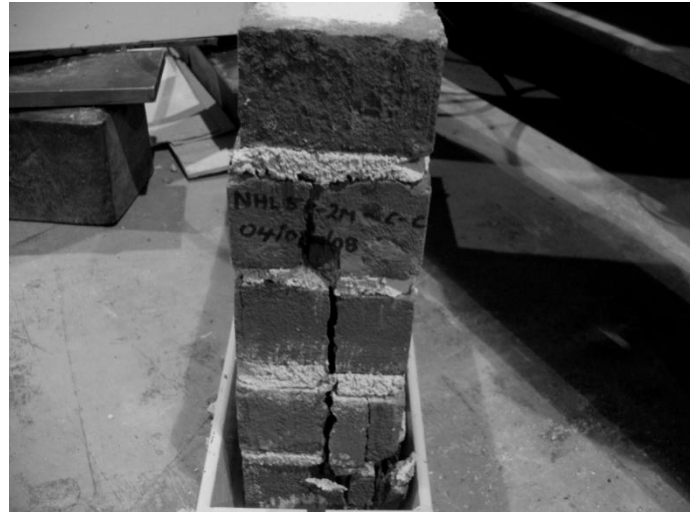
Figure 4 NHL 5 56 day compression test failure
