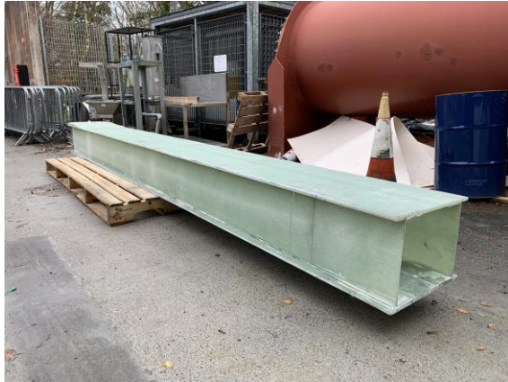
Figure 3: Demonstrator manufactured using glass fibre-reinforced composite materials
