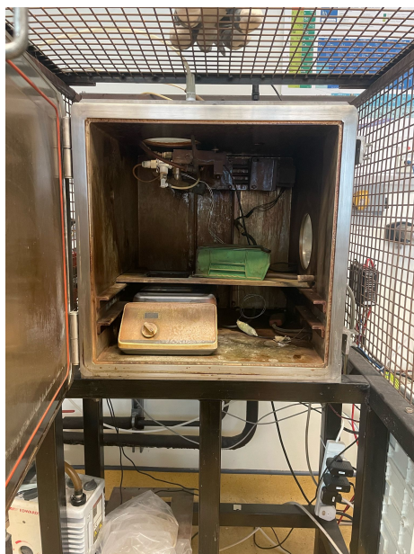
Figure 3.5: Image of the interior of the spray pyrolysis chamber used for growths of zinc-tin oxide samples
