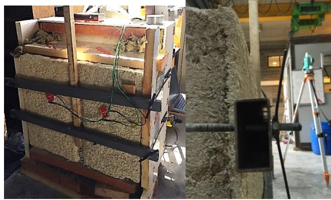
Fig. 2. Hot-box assemblage for thermal conductivity measurement.
