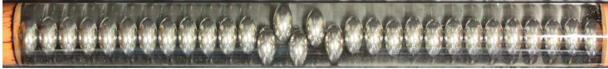
Fig. 7. Buckled chain of 30 steel spheres (diameter 6.32 mm) confined in a perspex cylinder (inner cylinder diameter 1.6 cm) and under compression, \Delta = 0.85 . The spheres, which are undeformed, are immersed in vegetable oil to reduce friction between them. (The presence of the oil leads to a large optical distortion; the measured ratio of lateral sphere extension to sphere diameter is about 1.9).
