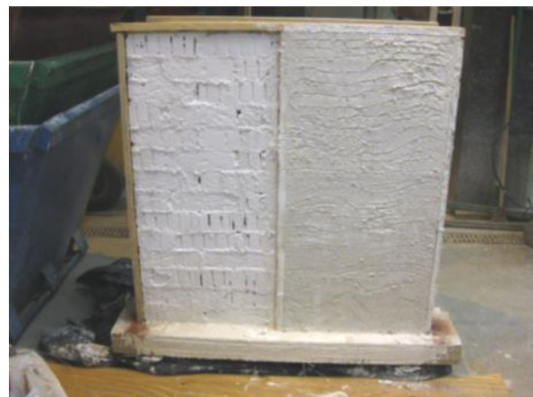
Fig. 1: A solid brick wall with hemp-lime render mix 5 applied.
